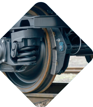
Backing plate = support of brake pad/lining
