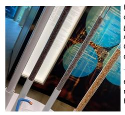
HEF's surface coating technology allows three successive coatings to be applied to these balls, with the final one being a gold finish. *"If we apply other finishes, we can access other markets that don't use the same soldering techniques", says* Guillaume Dubois, in charge of coated powder technology development.
